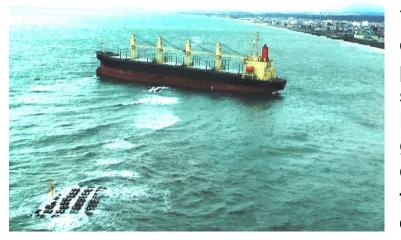
You should pay attention to dragging anchor in Kushiro port when a southerly strong wind is blowing. Dragging anchor leads to grounding or capsizing, and causes serious damage to the environment and the economy.
