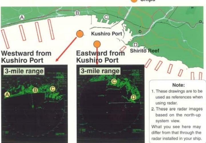
Radar reflectors are attached to the tips of stationary fishing nets, but it may become difficult to confirm these reflectors in the radar image depending on the weather. Please enter port by confirming the ship's location.
